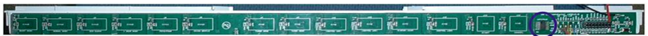
3. Cancellation of parasitic capacitances by differential sensing allows for long sensor traces.
