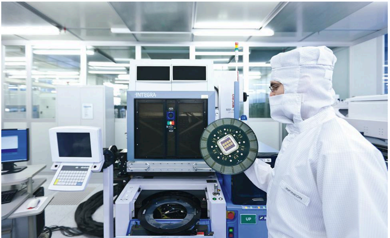
An Infineon Technologies engineer holds a 200 millimeter wafer in a semiconductor cleanroom in Dresden, Germany. (Image courtesy of Infineon)
